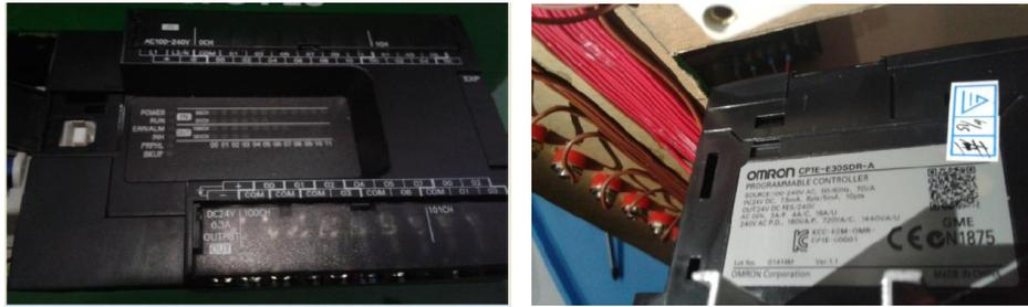
**Gambar 2.2 PLC Omron CP1E E30SDR-A**
