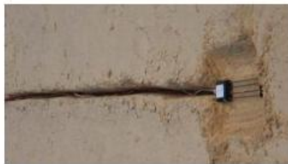
Figure 2.12. Installation of flat probe SMS
