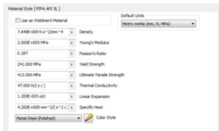
Gambar 4. 5 Material Properties API 5 L
