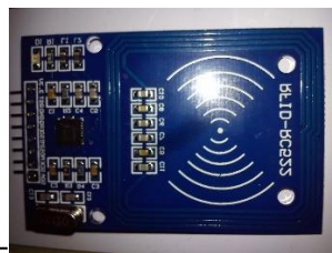
Gambar 2. 14. RFID reader RC522
