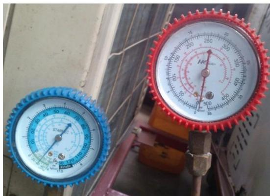
**Gambar 3.5.** *Pressure Gauge* – *Low Pressure* (biru), *High Pressure* (merah)
