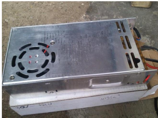
**Gambar 3.9.** *DC Power Supply* (Adaptor)
