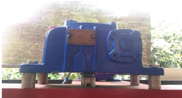
**Gambar 2.13 Transmisi (Gearbox)**
