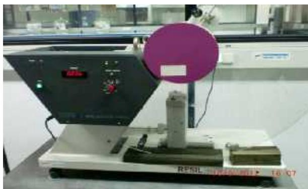
**Gambar 3.7** Mesin Uji Impak Resil Impactor
