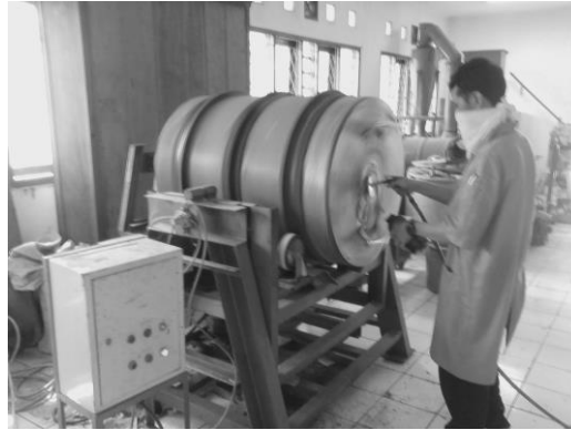
Gambar 3.4 Drum berputar ( Glue Mixing Drum )
