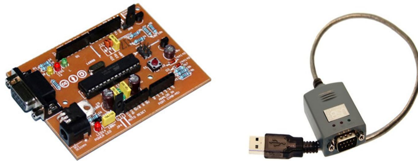
Gambar 2.23. (a) Arduino S3V.3 R2 (AT-Mega 8), (b) Konektor RS-232.
