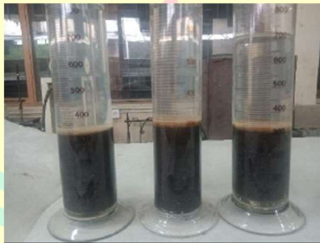
Hasil Pengujian Kadar Lumpur
