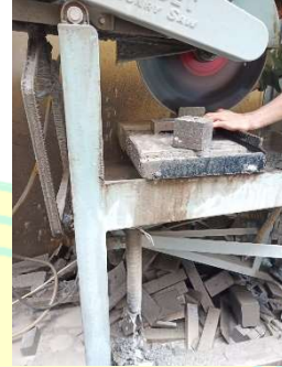
Proses pemotongan paving block
