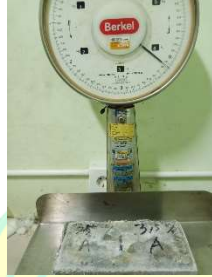
Proses penimbangan berat paving block
