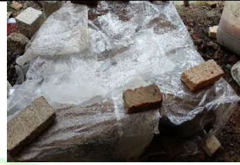
Proses Curing Benda Uji Balok
