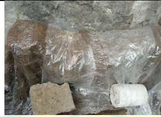
Proses Curing Benda Uji Silinder
