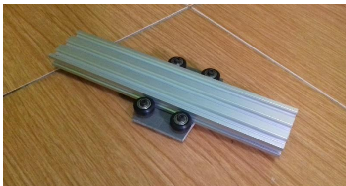
Gambar 2.12 Rel Aluminium Vending Machine
