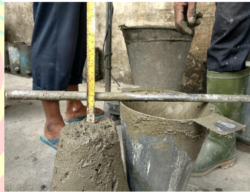
Beton Agregat FAPET 25% (48 mm)
