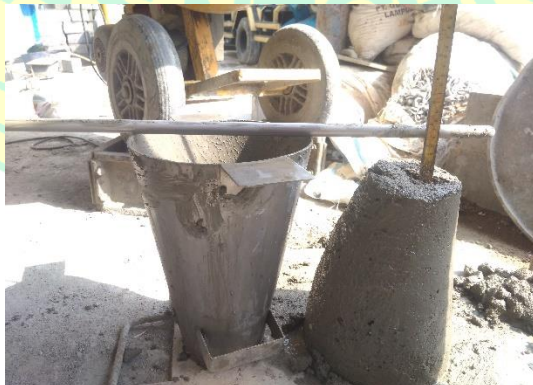
Beton Agregat FAPET 100% (60 mm)
