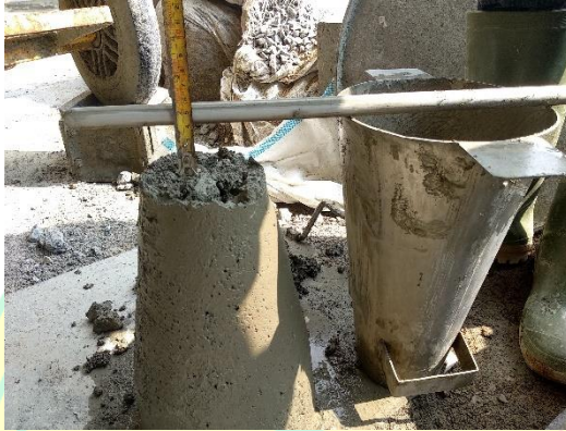
Beton Agregat FAPET 0% (45 mm)
