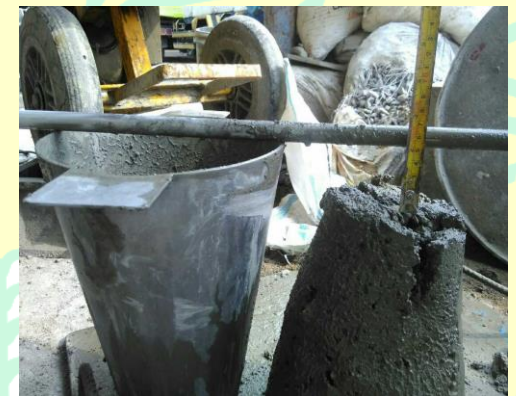
Beton Agregat FAPET 75% (56 mm)
