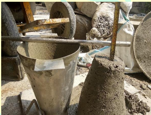
Beton Agregat FAPET 50% (50 mm)
