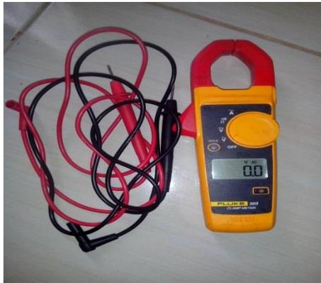
**Gambar 3.1 Alat Ukur Tang Ampere**
