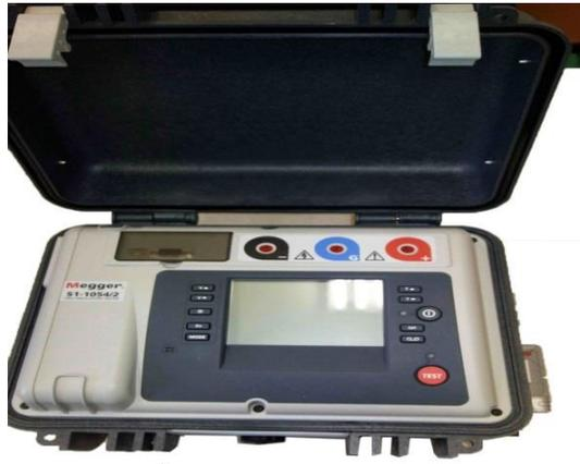
**Gambar 3.2 Alat Ukur Megaohm Meter**
