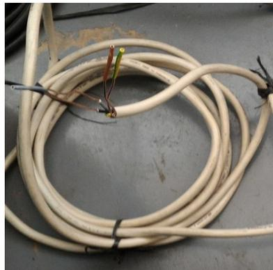
**Gambar 4.2 Sampel Kabel NYM 4 x 4 mm<sup>2</sup>**
