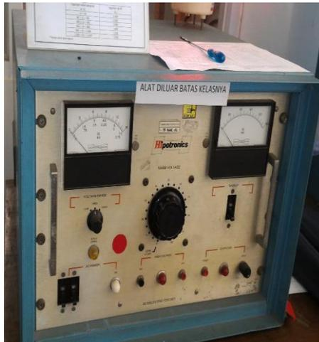
**Gambar 3.3 Alat Ukur HV Test**
