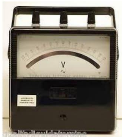
Gambar 9.26 Voltmeter Standard Multi Batas Ukur
