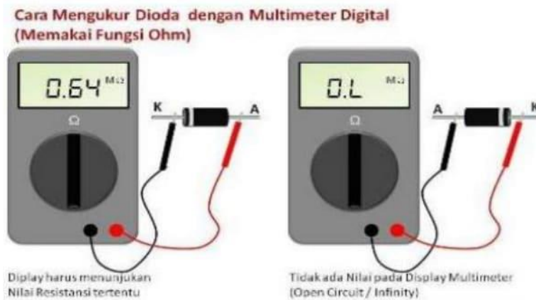
Gambar 5.5 Multimeter Pengetes Dioda
