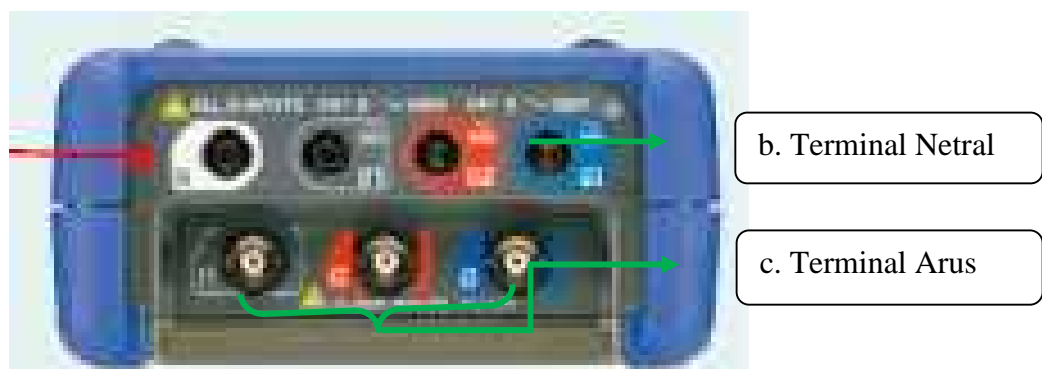
Gambar 3.1 Power Quality Analyzer HIOKI 3197 Tampak Atas
