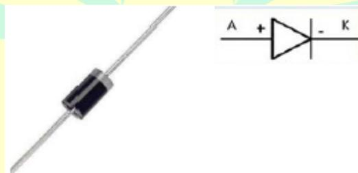
**Gambar 2.10 Diode (Kiri), Simbol Diode (Kanan)**
