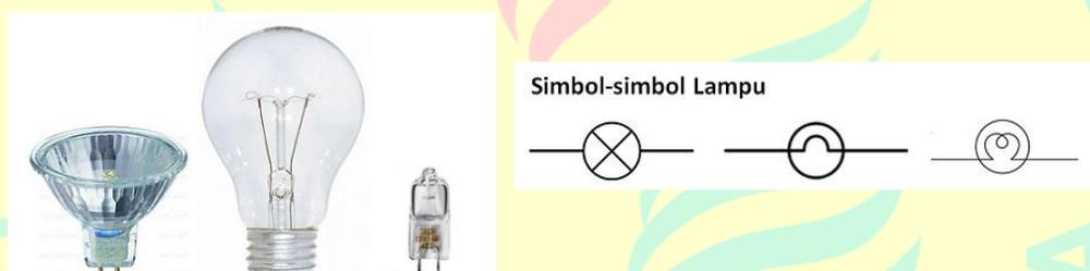
**Gambar 2.19 Lampu Indikator (Kiri), Simbol Lampu (Kanan)**
