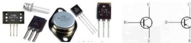
**Gambar 2.14 Transistor (Kiri), Simbol Transistor (Kanan)**
